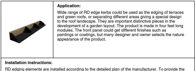
RD edging elements are installed according to the detailed plan of the manufacturer. To provide the continuity of water drainage, min. 2" thick base made up of mineral rubble with grain size of 1/8 - 3/8 " is applied on a heavy duty drainage layer (ex. DiaDrain-25H) on which the RDL kerb is placed after compressing and leveling the bedding. The edge elements are fixed to each other by screwing their endribs. Bulk material placed onto the base plate prevents the displacement of the structure.
