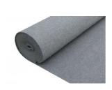
Diadem VLU-300 is a thermally-hardened, non-woven, needle punched fleece, intended to protect the waterproof membrane and retain storm water. The geotextile is resistant to bitumen and biological and chemical environments typically found in soils, and has limited resistance to UV degradation. Install on top of the root barrier layer or on root resistant waterproofing, end laps should be 12" and side laps 4".
