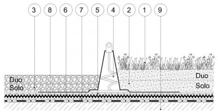
(1) Vegetation, (2) Growing media, (3) Gravel, (4) Dia Safe damping plate with integrated damping mat, (5)VLF-150/200 filter layer, (6)DiaDrain-25H flow-delay retention board, (7) VLU-300/500 mechanical protection layer, (8) Roof resistant waterproofing membrane, (9)Roof construction
