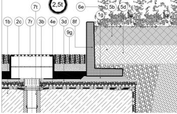
(8f)BW-80,(1g)Bedding,(6e)Vegetation,(5b)Growing media,(3d)VLF-200 filter layer,(4e)DiaDrain-40H,(3b)VLU-500 mechanical protection,(2c)Waterproofing membrane,(1b)Roof construction
