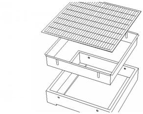
3-28-2011 We need to find a solution for fixing the grilles, and change the housing sizes for  $18{\times}18"$  and  $24{\times}24"$
